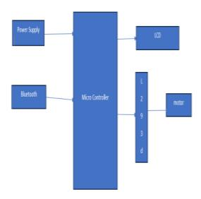
DC motor- 1 positive terminal is connected to pin-10 of Arduino and negative terminal is connected to pin -11 of Arduino. DC motor-2 positive terminal is connected to Arduino pin-9 and negative terminal is connected to Arduino pin-6. Two servo motors are use. One for performing sweeping operation and another one for performing the cleaning operation. It is controlled with Bluetooth via mobile phone. The servo motor-1 is coupled to the pin-5 of
